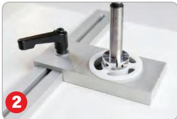
Drill light hole to desired depth using adjustable stop.
