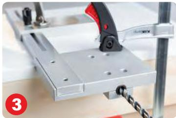
Leave clamps in place drill wire hole until bit reaches light hole.
