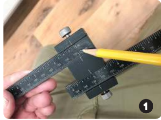
1 For fast repeatability use the Extended Ruler Attachment
