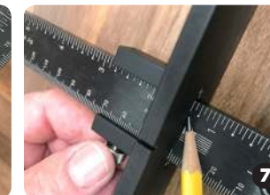
7 Match side measurement to Large Stop and tighten
