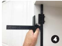
Slide two drill bushings side by side lining up center line with your mark
