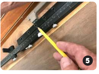
5 Lay the pull on the jig align with taped hole
