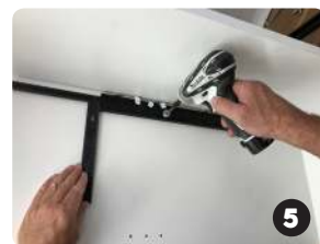
Remove Large Stop and press thumb screws against back panel then drill
