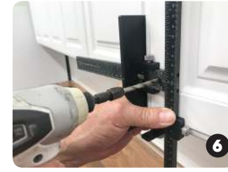
6 Position tool with stops as shown and drill hole through drill bushing
