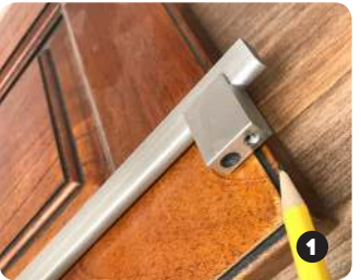
1 We demonstrate a method to center a long pull on a Drawer - line up center of one hole with edge of Drawer
