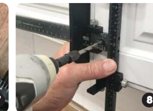
8 Position tool as shown drill through fixed center bushing for bottom hole
