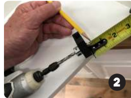
Set stop collar to drill depth
