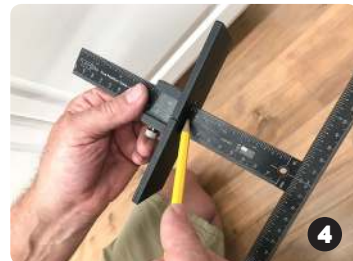
Slide Large Stop to match side measurement
