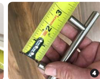
4 Measure hole centers of your hardware
