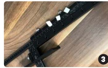
Mark your holes with tape for reference
