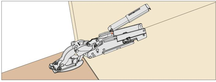
Lift the door slightly and snap the other end of the Smove into position. This operation is tool free.
