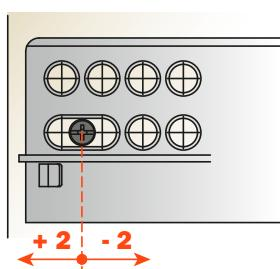
The oval slot allows the easy alignment of drawer frontals particularly in multi drawer and Push applications.
