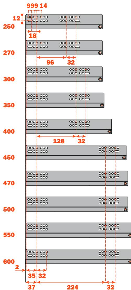
Detail of the rear additional fixing hole
