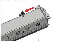
Insert the tilt adjustment levers, both right and left
