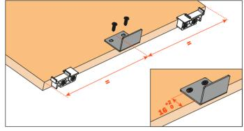
2) Fix the magnet to the bottom.
