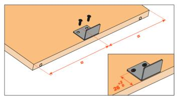
1 B) Fix the bracket to the shelf with the rear hook support. The bracket needs to be aligned to the rear hook support.
