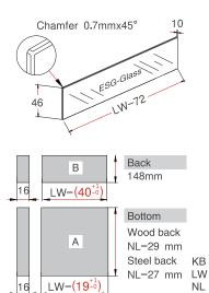
Chamfer 0.7mmx45° 10 ESG-Glass \_150 140 NL <n 40 = Cabinet Width
