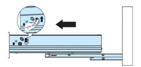
To re-install, place drawer on extended slides and push the drawer in fully. When it clicks, the lock will be engaged. Replace cover caps on both sides.
