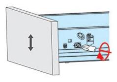
When finished with your adjustments, snap the cover caps back onto the drawer.
