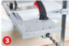
3 Leave clamps in place drill wire hole until bit reaches light hole.
