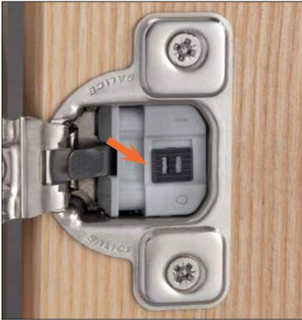
Switch dampening effect OFF by turning the lever to 0.
