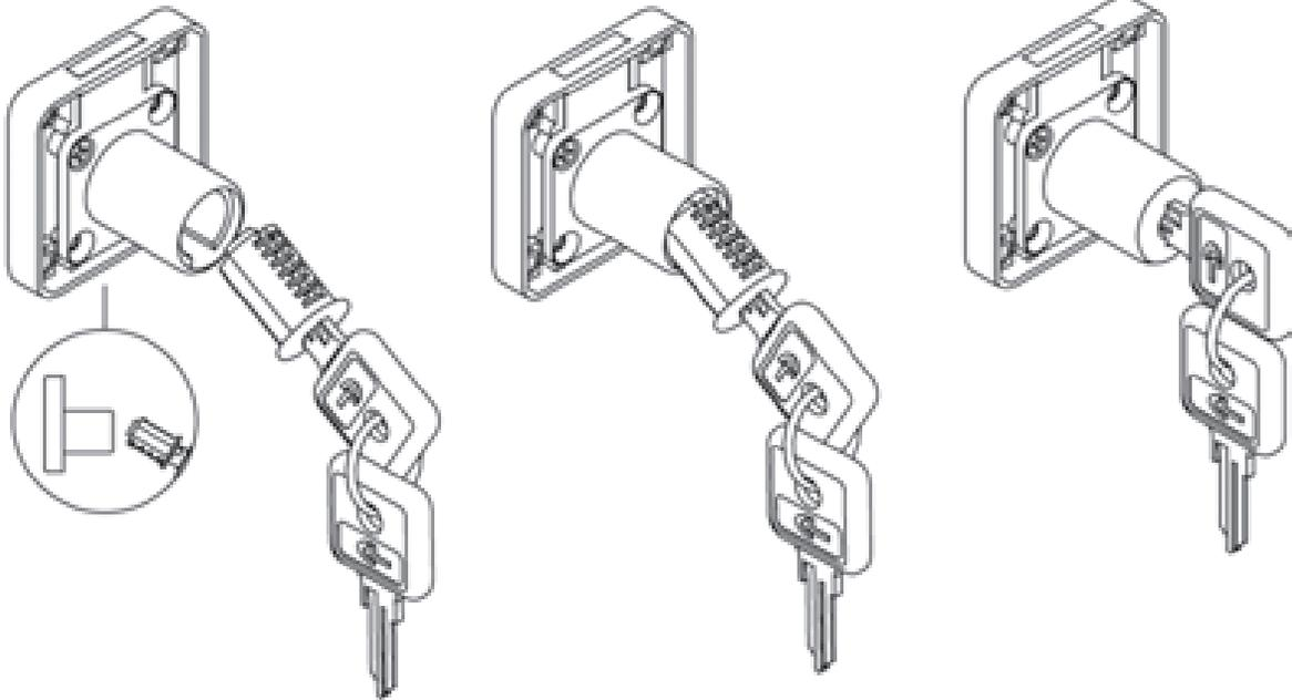
▶▶ **1 & 2** Install cylinder core with key inserted into the cylinder housing. Be sure to align the two diamond shaped objects on both the cylinder core and the cylinder housing.
