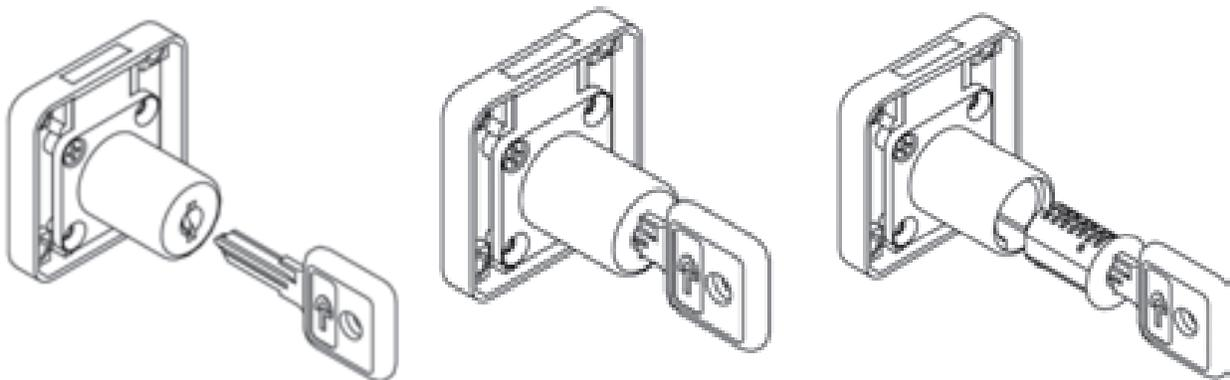
▶▶ **1 & 2** Insert removal key into cylinder core.
